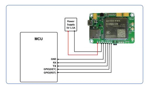
The 7SEMI LTE modem interfaced with Host/MCU using Main UART of Quectel EC200 .The main UART interface supports 9600bps, 19200bps, 38400bps, 57600bps, and 115200bps and 230400bps baud rates.
